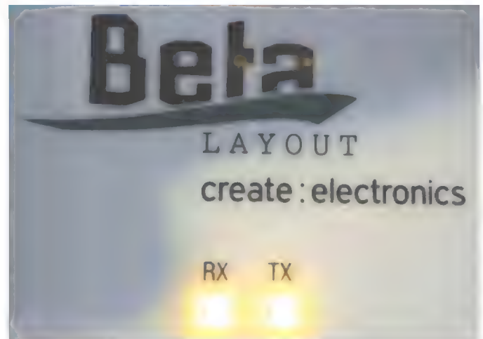
Figure 19. USB indicators. They illuminate when the controller is on.
